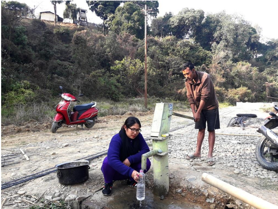
Plate 2b: Collecting water sample for analysis of physico-chemical and biological water parameters from handpump, Chandel district
